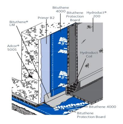
Details shown are typical illustrations only and not working drawings. For assistance with working drawings and additional technical advice please contact your local GCP representative
