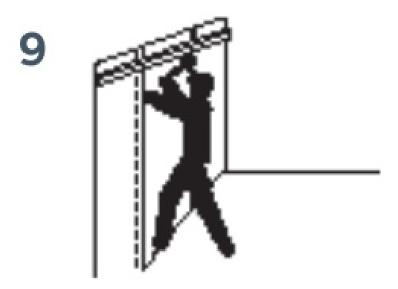
Where Bituthene is to be temporarily left exposed on vertical surfaces battening may be necessary to prevent slippage.
