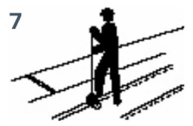
Roll all overlaps firmly with a Bituthene Lap Roller to ensure continuity of the Bituthene.
